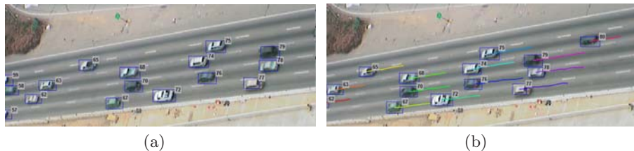
Fig. 1. Two frames (209, 218) of a traffic sequence are viewed in which the objects are identified and tracked
