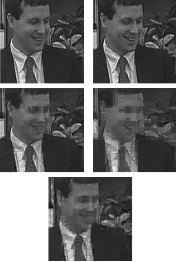
Fig. 12. Detail of the 855th frame of “Paris”: (a) original (20.2752 Mb/s), (b) PPCASOM compressed (4.2695 Mb/s), (c) SOMM compressed (4.4292 Mb/s), (d) KBTM compressed (2.2345 Mb/s), and (e) PCA compressed (4.7050 Mb/s).
