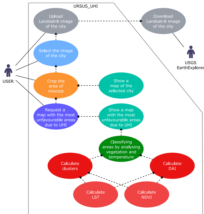
Fig. 2. Use case diagram. The following model describes the main functionalities of the system; both the internal functions and those offered to the user through the interface.
